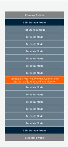
Figure. Teradata IntelliFlex platform cabinet components.
